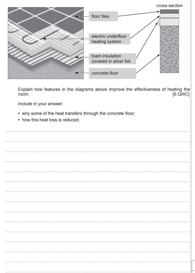
(c) The diagrams show how the underfloor heating system is laid under tiles.
